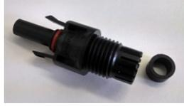
2. Strip end of cable approx.  $\frac{1}{4}$ " and mate it with the winged end of the pin or socket. Squeeze wings of Pin or Socket down to restrain the portion of wire that has been stripped. Then solder where the wings of the pin pinch the bare wire. Note: The insulation should not be inside the wings of the pin but should come fairly close to the wings.
