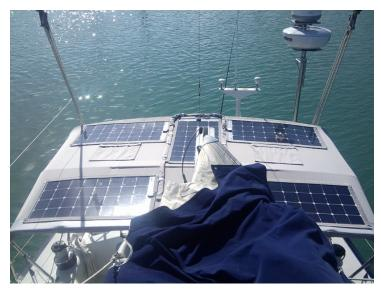
Note that the Velcro is both sewn and glued to the panel. Also note that in this case a bit more clearance could have been left between the Velcro and the cells to avoid shading the cells.
