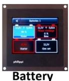
Displays volts, charge/discharge amps, capacity remaining in both percentage and amp/hrs, time remaining to alarm level at present current draw, alarm level, and temperature (with optional sensor). Each fully monitored battery has user-adjustable alarm thresholds for low capacity and requires a 300 or 600 amp continuous rated Shunt. Voltage of a second battery can also be displayed, with alarm capability.
