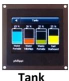
Displays liquid levels in four tanks in percentage and liters. Blue = water, yellow = fuel, gray = gray water, green = waste. User-adjustable alarm thresholds for either an emptying or filling tank, plus manual reset for a tank with Flow Meter. Requires one CMT for up to four tanks, and a tank sensor or flow meter for each tank. Use Ultra Sonic Tank Sensors UTV or Flow Meter DFS. Other types of sensors are supported.
