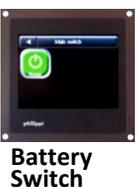
Remote Battery Switches are displayed and colored according to their status: green = operated, red = disconnected. Switches can be activated either from the Display, from a separate push-button or key switch, or in an emergency, on the switch itself. Low and high voltage disconnect thresholds are set on the PSM Display, together with password protection if desired. Requires FBC 260 Remote Battery Switch.
