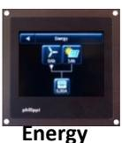
Displays charge and discharge currents for individual loads and charge devices, plus individual accumulative amp/hrs charged or consumed. Charge devices shown on top row (i.e. charger, solar, wind generator, etc), and consumers on bottom row (i.e. windlass, inverter, battery, etc.). Each device monitored requires a 300 or 600 amp continuous rated Shunt.
